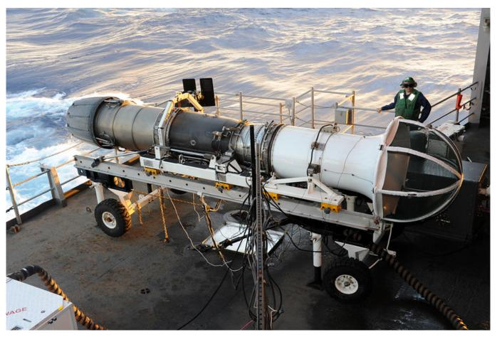
ATLANTIC OCEAN (July 16, 2011) Aviation Machinist's Mate Airman Matthew Kephart observes an F404-GE-402 jet engine on a test cell as it is fired up on the fantail aboard the aircraft carrier USS Dwight D. Eisenhower (CVN 69). Dwight D. Eisenhower is underway conducting carrier qualifications.(U.S. Navy photo by Mass Communication Specialist 3rd Class Nathan Parde/Released) 110716-N-AU622-029
