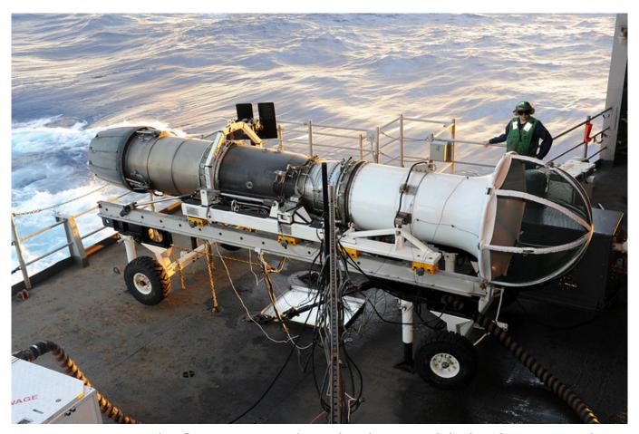
ATLANTIC OCEAN (July 16, 2011) Aviation Machinist's Mate Airman Matthew Kephart observes an F404-GE-402 jet engine on a test cell as it is fired up on the fantail aboard the aircraft carrier USS Dwight D. Eisenhower (CVN 69). Dwight D. Eisenhower is underway conducting carrier qualifications.(U.S. Navy photo
